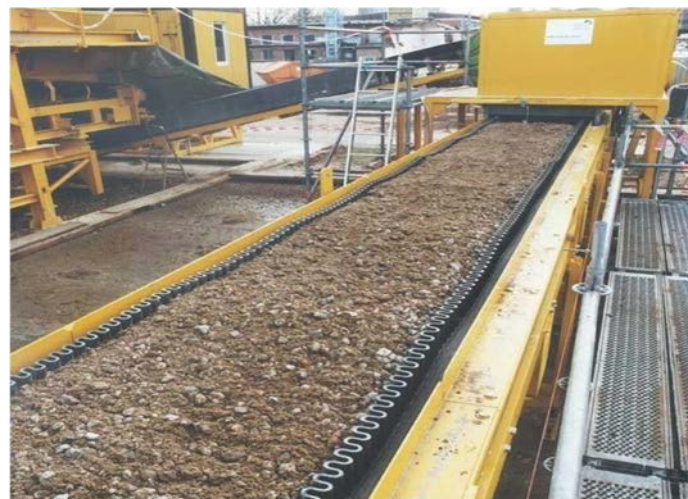
Figure 3: Conveyor belt monitor for free release of large amount of soil
