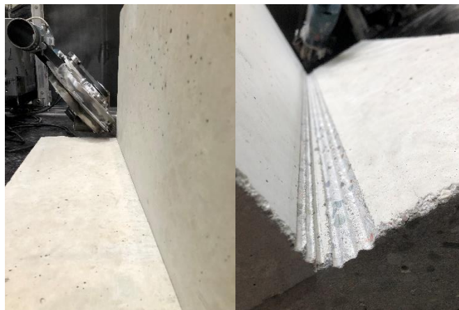
Figure 2: Tool to be tested in the tool holder (left) and concrete surface after the processing (right)
