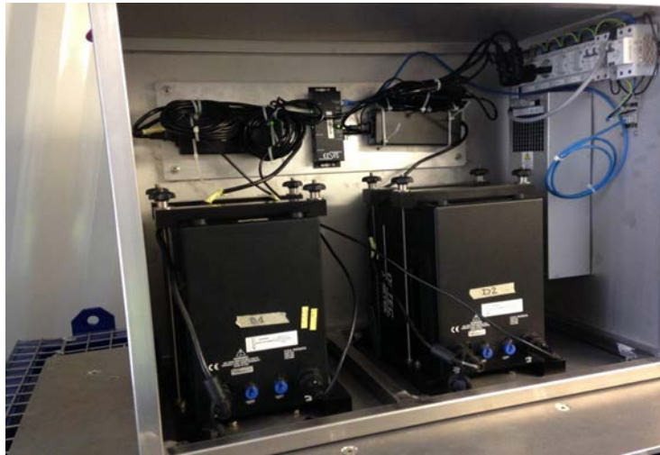
Figure 4: Measurement housing with array of electrical cooled HPGe spectrometer, mounted above the conveyor belt
