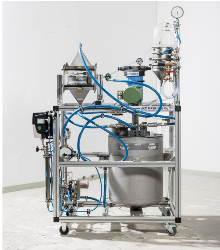
Figure 2: MASK separation test plant [1]
